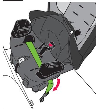
Pull the seat pad off of the front of the child restraint. Route the Lower Anchor Connector strap and hook through the rear-facing belt paths.
