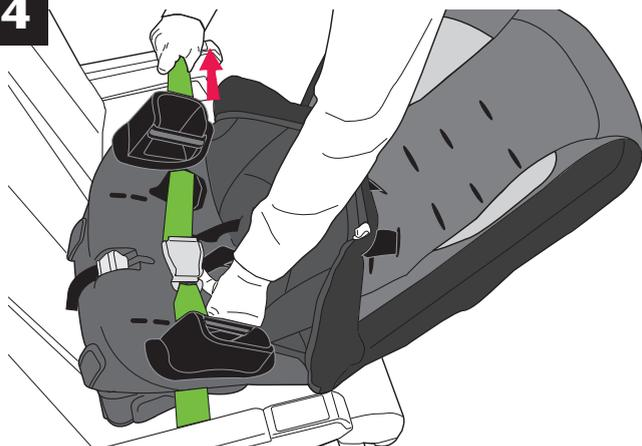
The aircraft seat belt must be as tight as possible. Route the excess seat belt strap back through the rear-facing belt path opening, as shown above. Using your full weight, push the child restraint firmly onto the aircraft seat while pulling on the excess seat belt strap to tighten.
