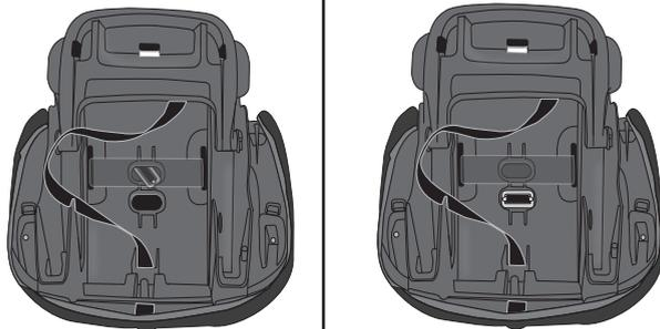
To reposition the crotch strap, first turn the child restraint upside down. Turn the crotch strap harness anchor sideways and push it through the slot in the bottom of the seat shell.
