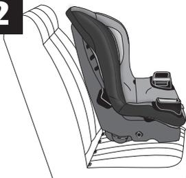
Adjust the child restraint to the **upright position** (page 44). Place the child restraint in your vehicle **forward-facing**. Unhook tether strap from the rear of the child restraint and place tether hook with **red adjuster** (p. 48) over back of vehicle seat.
