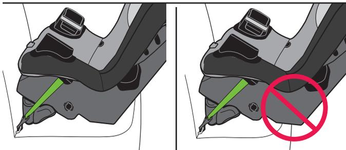
**Note:** When in rear-facing position, bottom of child restraint **MUST** be entirely on vehicle seat.
