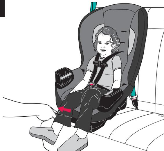
To tighten the harness straps, pull on the long harness adjuster strap on the front of the seat.
