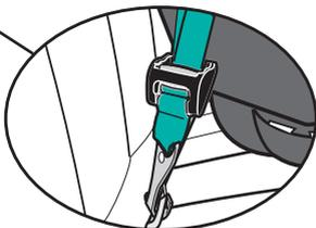
Tilt the adjuster and slide the strap to loosen.
