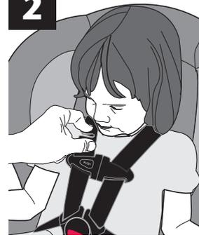
The harness straps must be snug against the child. A snug strap should not allow any slack. It lies in a relatively straight line without sagging. It does not press on the child's flesh or push the child's body into an unnatural position. Check the harness straps near the shoulders for slack. You should **NOT** be able to pinch the harness (see illustration). Adjust as needed.
