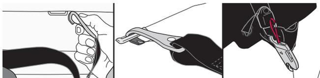
Refer to your vehicle owner's manual to locate the lower anchor bars on your vehicle seat. Attach the right hook, or clip, to the right anchor bar and the left hook, or clip, to the left anchor bar. **DOUBLE CHECK** that the lower anchor connector hook is fully engaged by pulling hard on the lower anchor connector strap.
