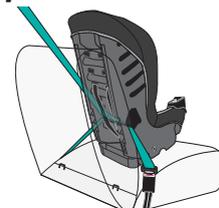
Fasten the vehicle seat belt as shown depending on your type of seat belt.
