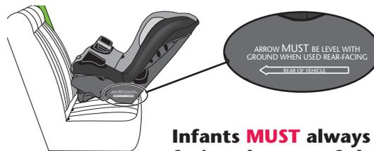
Adjust the child restraint to the **recline position** (page 44). Place the child restraint in your vehicle **rear-facing**. Adjust the restraint so that the level arrow is level with the ground.
