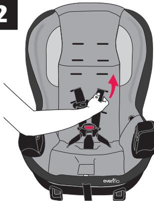
Pull harness strap through to the front of the child restraint. Thread each harness strap through the appropriate slot. Pull the harness strap to the back of the child restraint.
