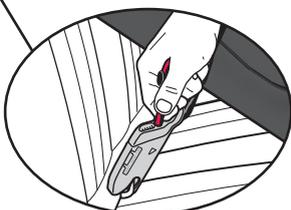
To remove the hook, press the tab and twist, then remove from anchor.
