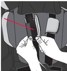
Install Harness Covers above Chest Clip. Harness covers are optional for added comfort. Wrap Harness Covers around harness straps and attach Velcro strips as shown.
