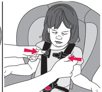
Fasten the chest clip by snapping the two halves together, as shown. Slide chest clip to armpit level.
