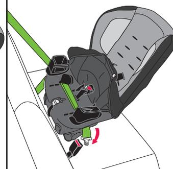
Pull the seat pad off of the front of the child restraint. Route the vehicle seat belt through the rear-facing belt path and continue through the opposite opening of the child restraint. **IMPORTANT:** Make sure the seat belt is **in front of the crotch strap**, and it lies flat without twisting, as shown. Fasten the vehicle seat belt, as shown, depending on your type of seat belt. Reconnect the seat pad to the front of the child restraint.
