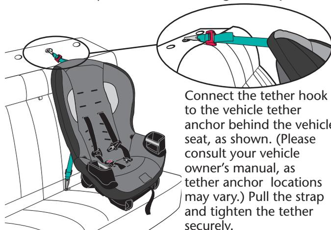
Connect the tether hook to the vehicle tether anchor behind the vehicle seat, as shown. (Please consult your vehicle owner's manual, as tether anchor locations may vary.) Pull the strap and tighten the tether securely.
