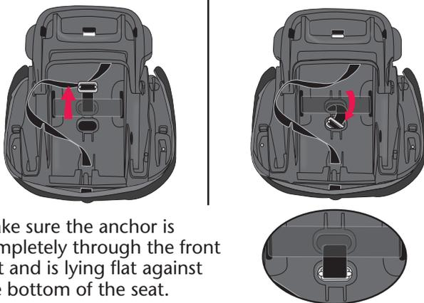
Make sure the anchor is completely through the front slot and is lying flat against the bottom of the seat.
