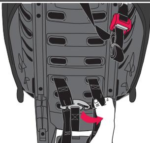
To change the harness strap position, loosen the shoulder harness as shown on page 47, step 2. Slide the harness strap off the splitter plate. We recommend doing this one side at a time
