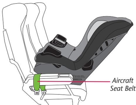
Adjust the child restraint to its **recline position** (page 44), then place it on the aircraft seat **rear-facing**, as shown above.
