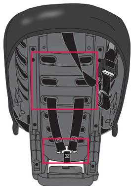
Make sure that the harness straps are in one of the **three upper** strap slots. The harness straps **MUST** start at shoulder height or above, using the strap slots closest to your child's shoulders. The splitter plate is attached to the bottom of the harness strap in the **child position** (page 43). This will provide more room for your child to fit comfortably.
