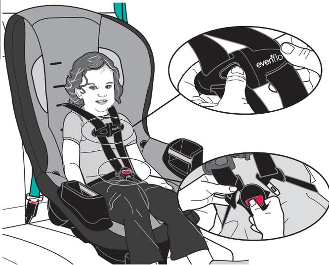
Push the release button and pull the chest clip apart. Press the red buckle release and remove the buckle tongues.
