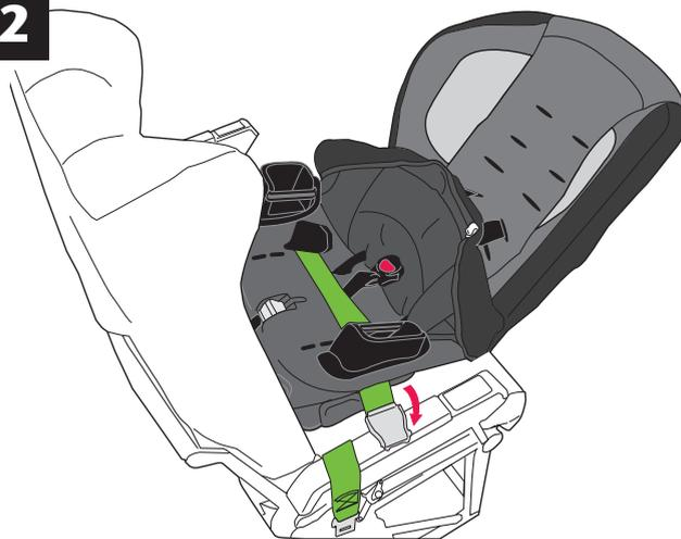
Pull the seat pad off the front of the child restraint. Route the aircraft seat belt through the rear-facing belt path opening on one side and continue through the belt path opening on the opposite side of the child restraint, as shown above.
