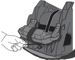
When the recline stand is in the recline position, wrap Velcro® strap around the recline stand and insert the end of the strap through the D-ring, as shown.
