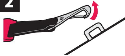
Press the tab and twist, then remove the hook from the anchor.
