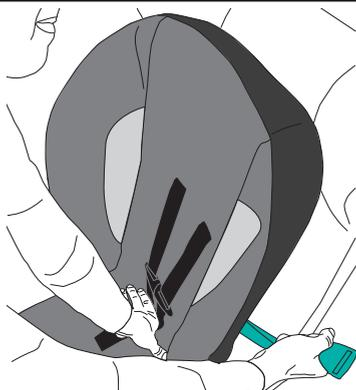
The aircraft seat belt must be as tight as possible. Route the excess aircraft seat belt strap back through the forward-facing belt path opening, as shown above. Using your full weight, push the child restraint firmly onto the aircraft seat while pulling on the excess seat belt strap to tighten.
