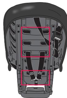
Make sure that the harness straps are in one of the **three upper** strap slots. The harness straps **MUST** start at shoulder height or above, using the strap slots closest to your child's shoulders. The splitter plate is attached to the bottom of the harness strap in the **child position** (page 43). This will provide more room for your child to fit comfortably.
