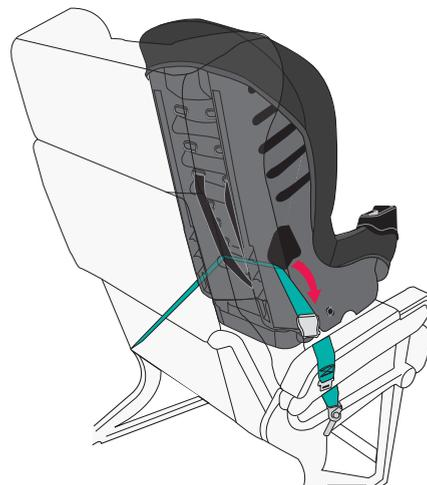
Route the aircraft seat belt through the forward-facing belt path opening in the back of the child restraint and continue through the belt path opening on the opposite side of the child restraint.
