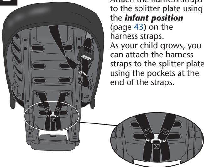
Attach the harness straps to the splitter plate using the **infant position** (page 43) on the harness straps. As your child grows, you can attach the harness straps to the splitter plate using the pockets at the end of the straps.
