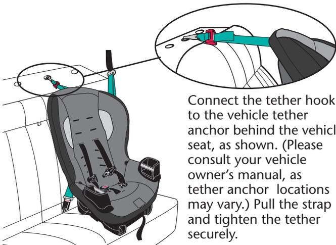
Connect the tether hook to the vehicle tether anchor behind the vehicle seat, as shown. (Please consult your vehicle owner's manual, as tether anchor locations may vary.) Pull the strap and tighten the tether securely.
