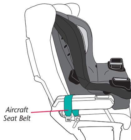
Adjust the child restraint to its **upright position** (page 44), then place it on the aircraft seat **forward-facing**, as shown above.
