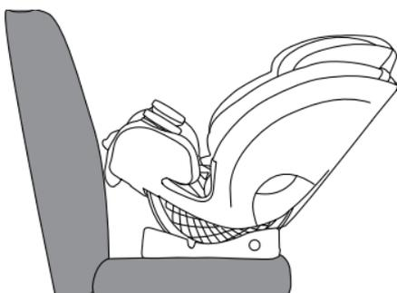
2. **Recline** child restraint to the appropriate position. Refer to page 15 to determine appropriate recline position.
