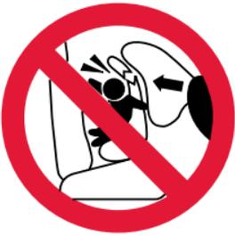
**DO NOT** place child seat rear-facing in the front seat of a vehicle with a passenger air bag. **DEATH** or **SERIOUS INJURY** can occur. Owners of vehicles with front passenger side airbags should refer to their owner's manual for child restraint installation instructions. The back seat is the safest place for children 12 and under.
