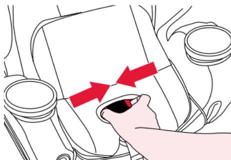
6. **Open** the storage pocket. **Remove** the lower connectors by pushing the red buttons and by pulling away from the child restraint.
