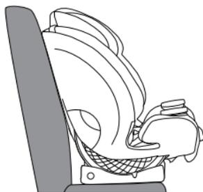
5. **Ensure** that no more than 3 in (7.6 cm) of the base hangs over the front edge of the vehicle seat.
