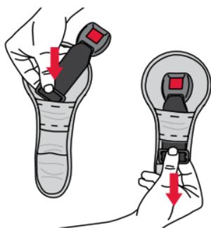
9. **Install** the buckle by turning its metal bracket sideways and routing it through the desired seat cover and CLICKTIGHT door slot. Refer to adjusting buckle position page 13.
