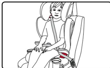
5. Route the lap part of the vehicle seat belt through the SecureGuard clip.
