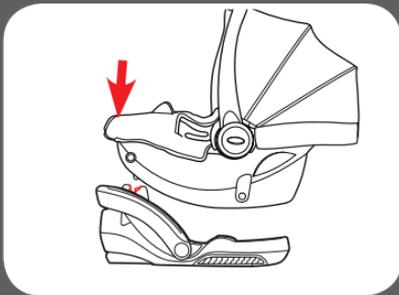
Pull up on the front corners of the seat to make sure it is locked.
