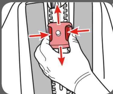
Move the head support up or down to the proper harness height position.
