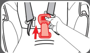
To clean, place in a cup of warm water and gently agitate the buckle. Press the red button several times while in the water.
