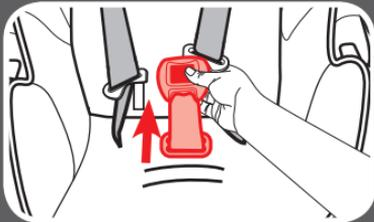
From the front, pull buckle out of the pad and shell.
