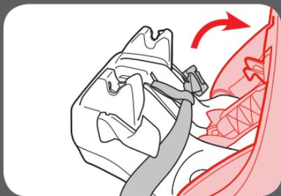
Swing open the LATCH storage door, and insert the LATCH connectors into the storage slots. Tuck the LATCH straps into the storage compartment and close the storage door.
