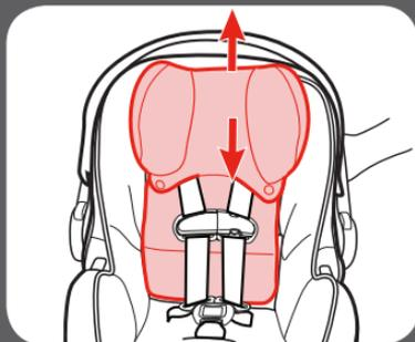
For smaller babies, shorten head support by placing the bottom of the flap under the support as shown.
