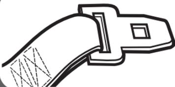
Grab the sides of the seat at the belt path and slide side to side and front to back. The base or seat should not move more than 1" (2.5 cm).
