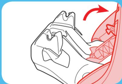
Swing open the LATCH storage door, and pull out the LATCH connectors.
