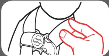
A snug harness should not allow any slack. It lies in a relatively straight line without sagging. It does not press on the child's flesh or push the child's body into an unnatural position.
