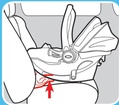
If needed, rolled towels may be placed under the base, at the vehicle seat crease, until the level line is level with the ground.
