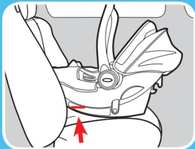
Check the rear-facing level line. The red level line on the side of the seat **MUST BE LEVEL** with the ground.
