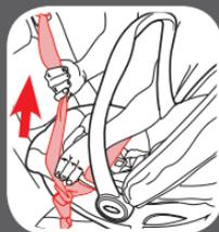
**Note:** With the vehicle seat belt in this locking mode, all the tension is upwards in the shoulder belt. This may start to tilt your car seat sideways when rear-facing. If this happens, use a locking clip instead of switching the retractor. See Sliding Latch Plate and ELR Retractor.
