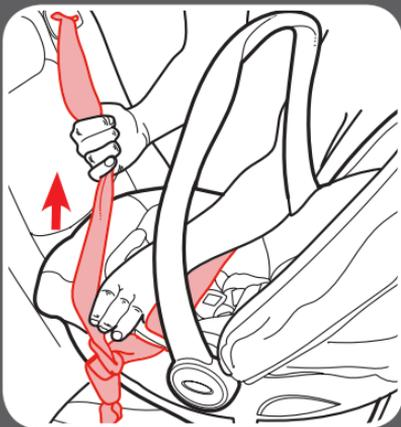
**Note:** When using the base, remove all the slack from the seat belt. The lock-off locks the seat belt.
