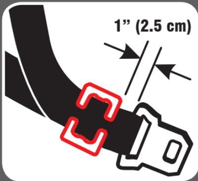
**Note:** When using the base, you do not need to use the locking clip. The lock-off locks the seat belt.
